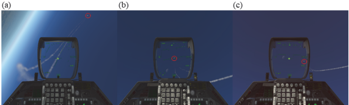
Fig. 6. Virtual simulation capture (a) Lag pursuit identified by the flight cloud (b) pure pursuit (c) lead pursuit
